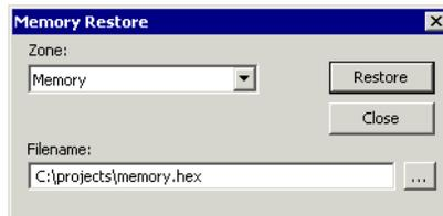
Use this dialog box to load the contents of a file in Intel-extended or Motorola S-record format to a specified memory zone.
