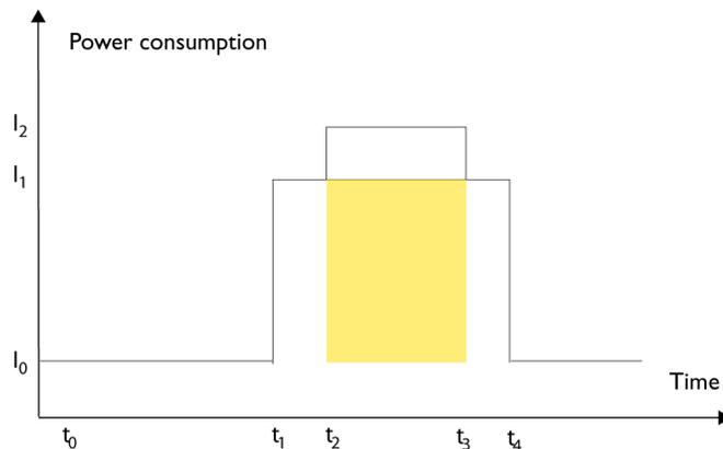
At  $t_1$ , the system is activated whereby the current rises to  $I_1$  which is the system's power consumption in active mode when at least one peripheral device turned on, causing the
