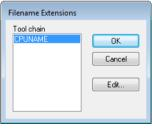
Use this dialog box to customize the filename extensions recognized by the build tools. This is useful if you have many source files with different filename extensions.
