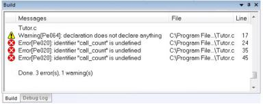
This window displays the messages generated when building a build configuration. When opened, the window is, by default, grouped together with the other message windows. Double-click a message in the **Build** window to open the appropriate file for editing, with the insertion point at the correct position.
