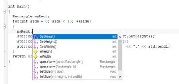
To insert a suggestion, either click it or select it with the arrow keys, and press Enter. To close the code completion pop-up window without inserting anything, press Esc.
