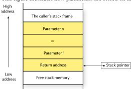
This figure illustrates how parameters are stored on the stack:
