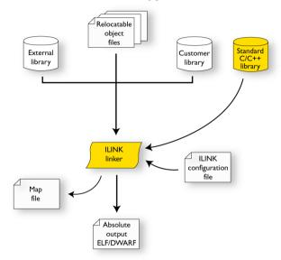
During the linking, ILINK might produce error and logging messages on stdout and stderr. The log messages are useful for understanding why an application was linked as it was. For example, why a module or section (or section fragment) was included.
