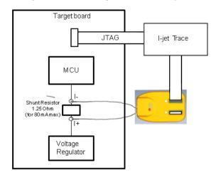
This figure shows how I-scope is connected to I-jet Trace and to the target board:
