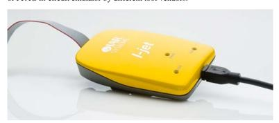
I-jet streams the program counter, variables, and power measurement data to the host computer to provide a view into program execution in real time. Besides the typical JTAG debugging, I-jet is capable of providing power to the target board and measuring it with sufficient accuracy to provide a power profile during program execution in real time. This feature is referred to as *power debugging*.
