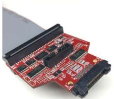
The mating connector for Mictor-38 on target board is AMP/Tyco 5767054-1.
