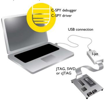
I-jet communicates using USB 2.0. (USB 1.0 is also supported but not recommended.) The I-jet in-circuit debugging probe is also referred to as a debug probe, debug adapter, or JTAG in-circuit emulator by different tool vendors.
