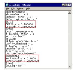
Save the settings file and restart the debug session. Open the J-Link Control Panel and verify that the "MemMap" tab shows the new settings for CFI flash and work RAM area.
