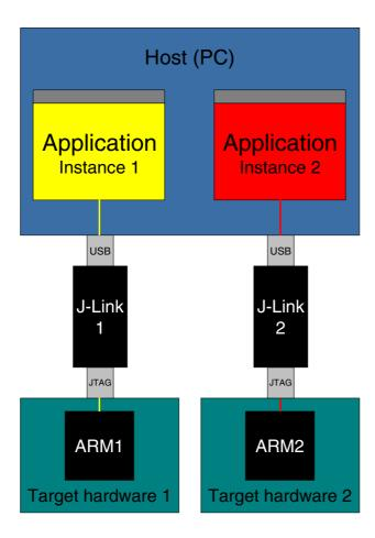
Older J-Links / J-Traces all reported the same serial number which made it necessary to configure them for USB0-3 if multiple J-Link should be connected to the same PC in parallel.
