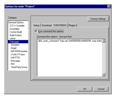
With these additional commands are the values of the fast GPIO registers in the C-SPY debugger correct and can be used for debugging. For more information about J-Link command line options refer to subchapter Command strings on page 75.
