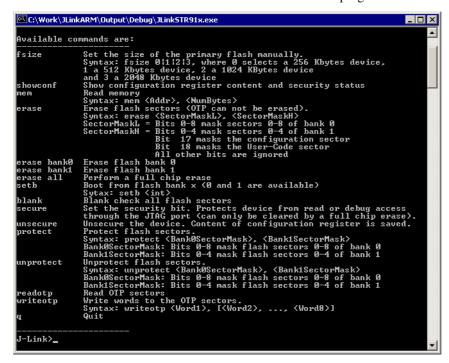
When starting the STR91x commander, a command sequence will be performed which brings MCU into Turbo Mode.
