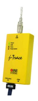
J-Trace for Cortex-M is a JTAG/SWD emulator designed for Cortex-M cores which include trace (ETM) support. J-Trace for Cortex-M can also be used as a regular J-Link and it also supports ARM7/9 cores. Please note that tracing on ARM7/9 targets is not supported by J-Trace for Cortex-M. In order to use ETM trace on ARM7/9 targets, a J-Trace is needed.
