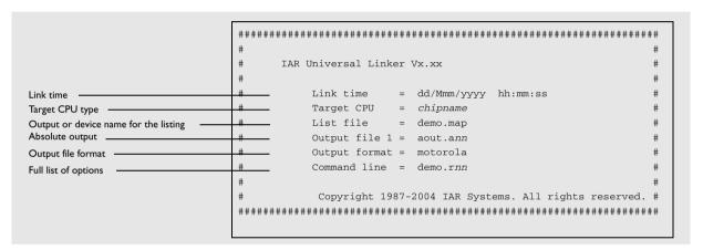
The full list of options shows the options specified on the command line. Options in command files specified with the -f option are also shown, in brackets.
