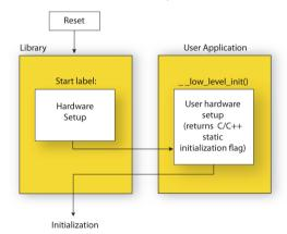
When the CPU is reset it will start executing at the program entry label \_\_program\_start in the system startup code.
