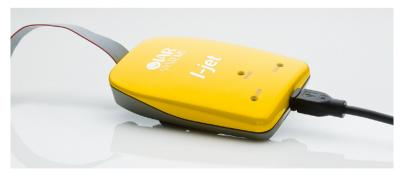
I-jet streams power measurement data to the host computer to provide a view into program execution in real time. Besides the typical JTAG debugging, I-jet is capable of providing power to the target board and measuring it with sufficient accuracy to provide a power profile during program execution in real time. This feature is referred to as *power debugging*.
