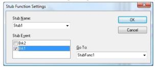
Use this dialog box to execute a stub function of the application on the occurrence of an event. The supported events are data accesses and execution events. Events that occur before execution cannot define a stub function call.
