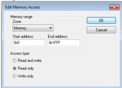
Use this dialog box to specify your memory address ranges for which you want to detect illegal accesses during the simulation, and assign an access type to each range.
