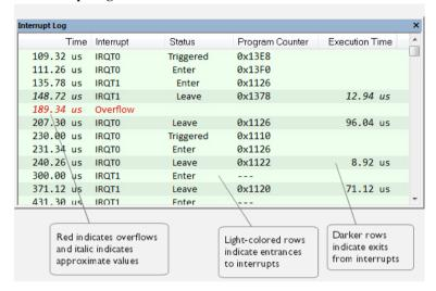
This window logs entrances to and exits from interrupts. The C-SPY simulator also logs internal state changes.
