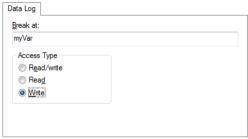
Use the **Data Log** breakpoints dialog box to set a maximum of four data log breakpoints on memory addresses, see *Setting breakpoints using the dialog box*, page 131.
